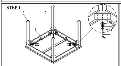
With the help of another person, place the table top (1) upside down on a clean, smooth surface. Attach the Table Leg (2) to the table top (1) with bolt (B), spring washer (D) and flat washer (E). Use the Allen Key (F) to tighten bolts (B). Repeat for all 4 legs
