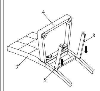
Insert the left and right stretchers (8 & 9) into the back frame (3) as shown above.
