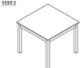
Turn the table upright on even surface. Tighten all screws and bolts. Use Allen Key provided.
