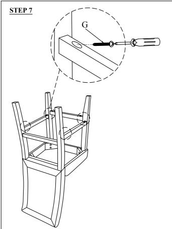
Attach the stretcher (7 & 8 & 9) to chair leg (5 & 6) and chair back leg (3) with screw (G) . Use the Phillips screwdriver (not provided) to tighten screw (G).
